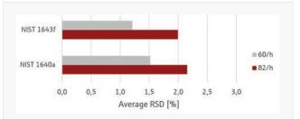
Drinking water analysis according to U.S. EPA 200.8. RSD of certified reference materials were measured with two different speeds. The outstanding sensitivity allows to measure >80 water samples per hour with competitive precision.
