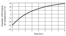
Conditions: AT 35°C, no load, measured at center of chamber
