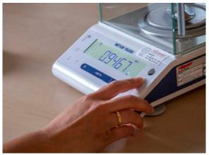
TRANSFER WEIGHTS FROM THE BALANCE TO LABCONNECT BY PRESSING A BUTTON. THIS WILL SAVE TIME.
