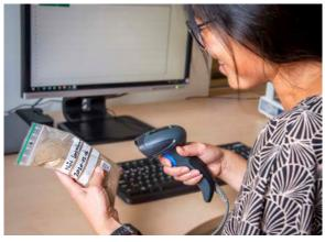
Connect a barcode scanner to LabConnect and use this when registering your samples. This will reduce errors and save time.
